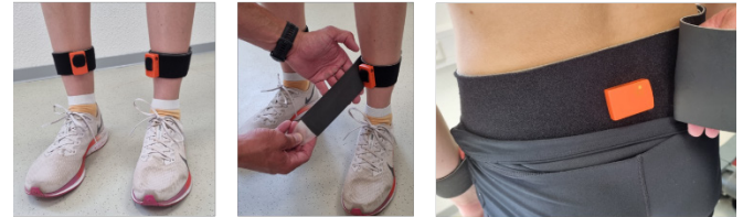
Figure 1: Experimental setup: Inertial measurement units were attached to the tibiae (and the sacrum) to measure triaxial peak accelerations.
