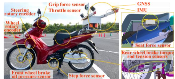
Figure 1: Motion capture system for motorcycle and rider.
