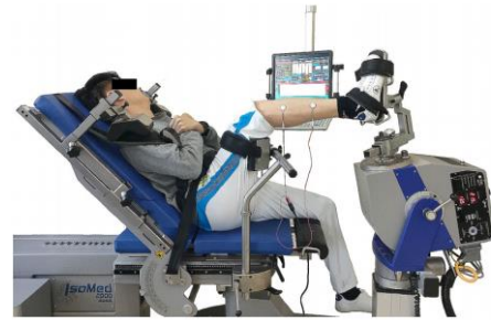
Figure 1: Illustration of superimposed-burst test in peroneal muscles
