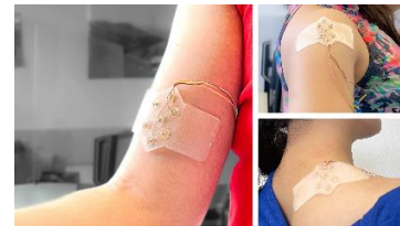
Figure 2: Application of the self-adhesive reusable electrode for the detection of muscular activation of different muscles.
